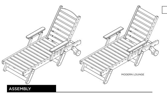
**STEP 1.** Use (8) 2" screws to attach spreader bars to front, center and wheeled back legs.
