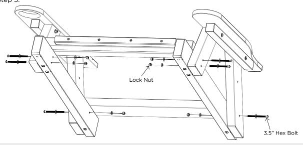
**STEP 2.** Position an upright as shown and secure it with a 3.5" Hex Bolt, a washer on each side of the material and a locknut. Repeat for the other side.
