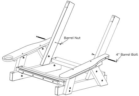
**STEP 4.** Using (2) 4.5" Barrel Bolts thread each through the bottom hole of the roll-up into the bottom hole of the upright as shown and secure using Barrel Nuts.
