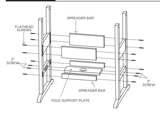
**STEP 1.** Insert Spreader Bars and pole support plate in place and use (12) 3" screws to attach to leg assemblies.
