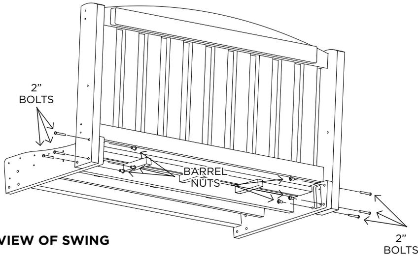
**STEP 3.** Use (6) 2" Bolts, and (6) Barrel Nuts to attach bottom of arms to bench.
