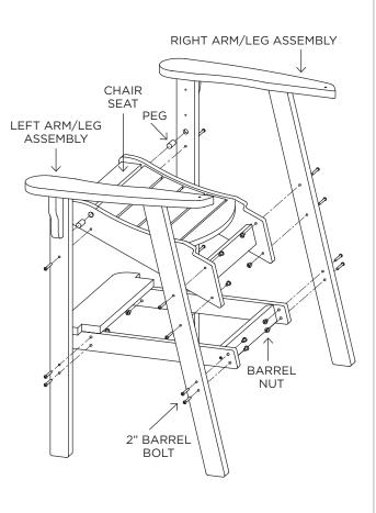
**STEP 3.** Use (2) 1.5" barrel bolts and (2) barrel nuts to attach chair back to right & left arm/ leg assembly.
