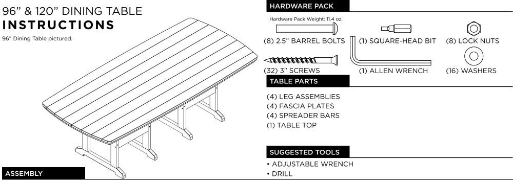
STEP 1. Use (16) 3" screws to attach fascia plates and spreaders to leg assemblies, repeat.
