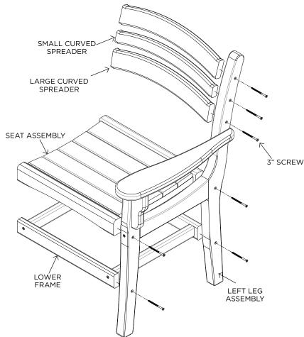
**STEP 2.** Use (7) 3" screws to attach the Right Leg Assembly to the Seat Assembly, Lower Frame, and spreaders.
