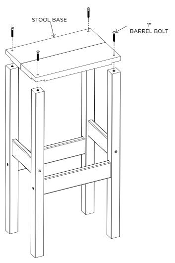
**STEP 3.** Place Stool Seat on top of the Stool Base, use (4) 1-5/8" Screws into pre-drilled holes to connect, and enjoy!
