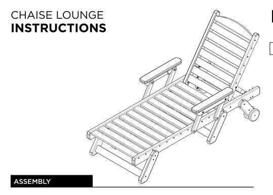
**STEP 1.** Use (8) 2" screws to attach spreader bars to front, center and wheeled back legs.
