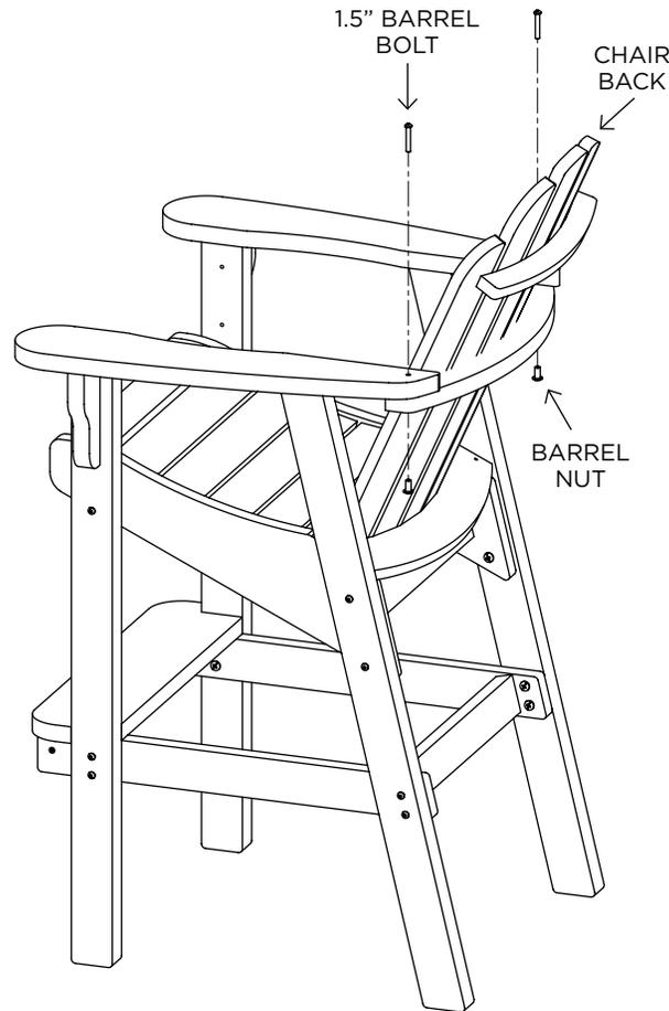
**STEP 4.** Use (2) 2" screws to attach chair back to chair seat. Tighten all bolts once screws are in.
