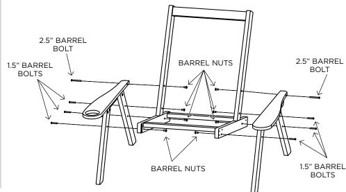
**STEP 3.** Use (4) 1.5" barrel bolts and (4) barrel nuts to attach rockers to legs. **Tighten all bolts.**
