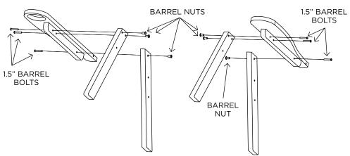
**STEP 2.** Use (2) 2.5" barrel bolts, (6) 1.5" barrel bolts, and (8) barrel nuts to attach arm assemblies & supports to inside of chair frame. **NOTE.** Do **not** tighten bolts until step 3.
