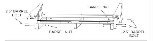
**STEP 3.** Use (2) 2.5" barrel bolts and (2) barrel nuts to attach frame to left and right supports. Use (2) 3" barrel bolts and (2) barrel nuts to attach left and right uprights to arms.
