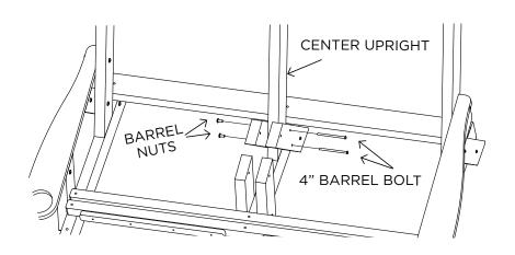
**STEP 6.** Attach (4) 4.5" barrel bolts, (4) barrel nuts in center beam. **(Eye bolts go on outsides)** Attach chain set to top of uprights using (2) 5.5" eyebolts (short chain) and to front of frame using (2) 4" eyebolts (long chain). Tighten all barrel bolt assemblies and nuts on chain set.
